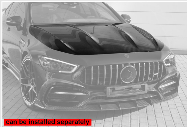
5. The hood is assembled from 4 parts
